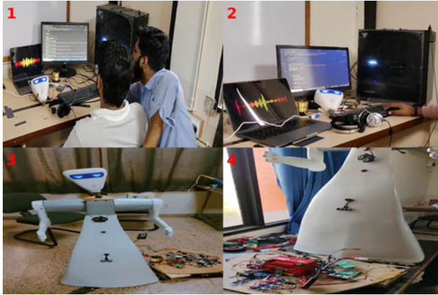
Figure 6. Experimental setup of the proposed system: (1) Hardware integration with robotic components for voice acquisition and task execution, (2) Testing and interface debug with voice signal visualization, (3) Prototype robot design for interaction and navigation, and (4) microcontroller and sensor setup for real-time operation and processing.
