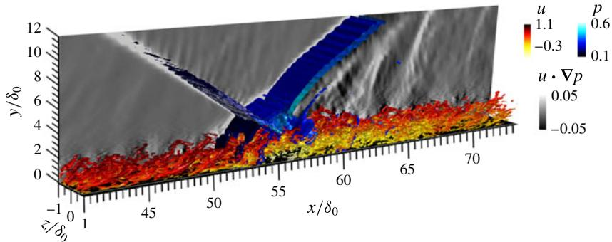
FIGURE 4. (Colour online) STBLI base flow: instantaneous isosurfaces of the  $Q$ -criterion coloured by streamwise velocity highlight hairpin vortices. The shocks (in blue) and background shading are indicated by an isosurface and contours of  $\mathbf{u} \cdot \nabla p$ .
