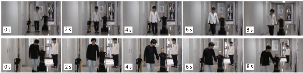
Figure 18. Time series photographs of the android that autonomously moves hand in hand with a human.
