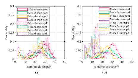
**Figure 12.** Probability histogram of the sum of squared mode shapes that belong to: (a) Training dataset of truss population 1 and testing dataset of truss population 1; (b) training dataset of truss population 1 and testing dataset of truss population 2.
