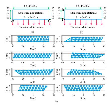
**Figure 4.** Visualization of the two generated datasets: (a) Geometric configuration meant to approximate a simply-supported truss population; (b) geometric configuration serving to approximate a cantilevered truss population; (c) some representative truss samples from the two datasets (only nodes and elements are displayed).
