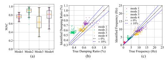
Figure 11. Performance of the trained model on the cantilevered truss dataset: (a) Box plot of MAC values of identified mode shapes; (b) scatter plot of identified damping ratios; (c) and scatter plot of identified natural frequencies.
