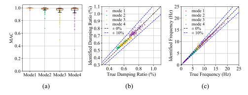
Figure 7. Performance of the trained model on the testing set of truss population 1 (simply supported):
