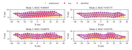
Figure 10. Mode shape identification results of a truss from the cantilevered population.
