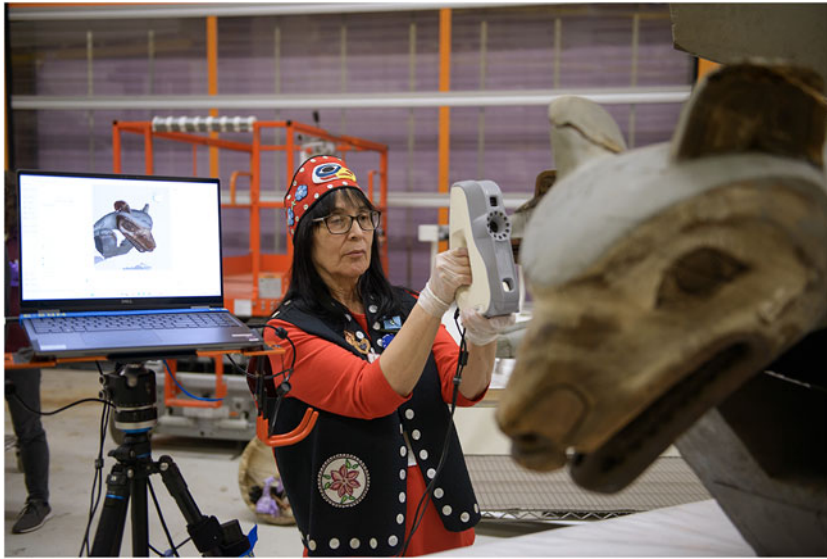
Figure 5. Tlingit Stax'héen Tláa (Stikine Mother) Luella Knapp, of the Naanyaa.ayi clan, using a structured light 3D scanner at the Smithsonian's Museum Support Center to digitize the prow of a 13.7 m long Brown Bear Canoe that belonged to the Naanyaa.ayi clan, whose spokesman was Chief Shakes. (Photograph by Walter Larrimore.)
