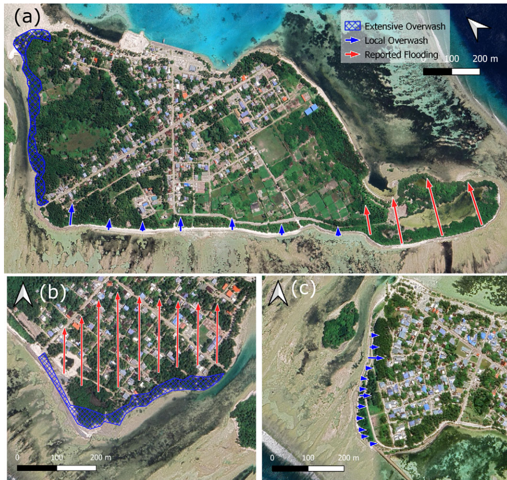
Figure 6. Mapped extent of island flooding and overwash deposits recorded after 1 July flooding event: (a) Fiyoaree; (b) SE margin of Rathafandhoo; and (c) SW margin of Fares-Maathoda. See Figure 1c for the location of the three atoll islands. Source: GoogleMap.
